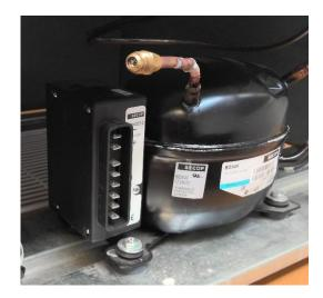
Step 5) Screw in ECU screw(clockwise). This will allow you to take off the ECU without taking off the screw.
