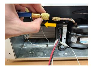
Step 17) Unscrew can from hose. Store the refrigerant in a safe place.
