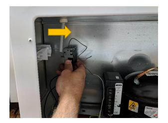
Step 6) Remove wires from thermostat with needle nose pliers. Grab by the connector.
