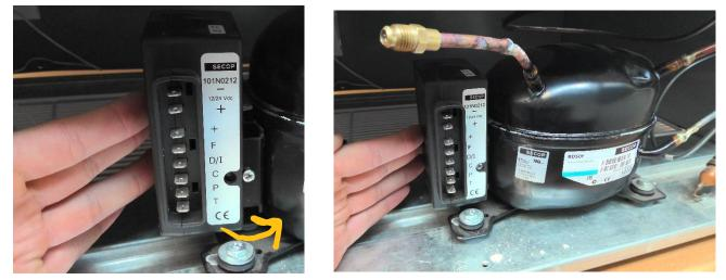
Step 11) Screw out ECU screw to fasten the ECU to the compressor. (Counterclockwise)
