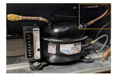
The suction line is where the refrigerant is returned to the compressor. If the system is overcharged the suction line will feel very cold. It may have frost on the outside. When the refrigerator is charged correctly, the suction line feels cool to the touch (think refrigerator temperatures). When the system is charged too little, then the suction line will be warm
